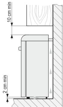
• The appliance must stand on a level surface and must not touch the wall. If necessary, regulate the height of the appliance by adjusting the levelling feet: by turning them clockwise – the front of the appliance rises, by turning them counter clockwise – it comes down. If the appliance is tilted slightly backward – the doors will close by themselves.
