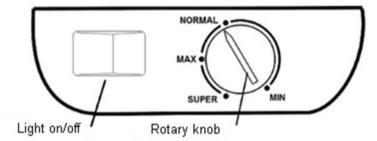
The thermostat has been adjusted using the temperature in the factory. Rotary knob a SET to raise or lower the temperature 0-10°C. Adjust the temperature according to usage, excessive cooling will increase unnecessary power consumption.
