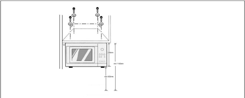
6. Connect the microwave to the floor of the cupboard with 4 screws and washers.
